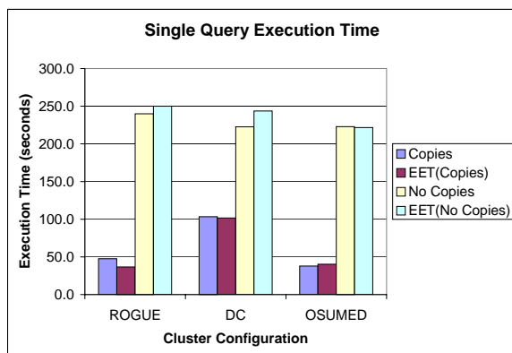
Figure 6: Single query execution time with and without copies. EET is the estimated execution time by the scheduler.
